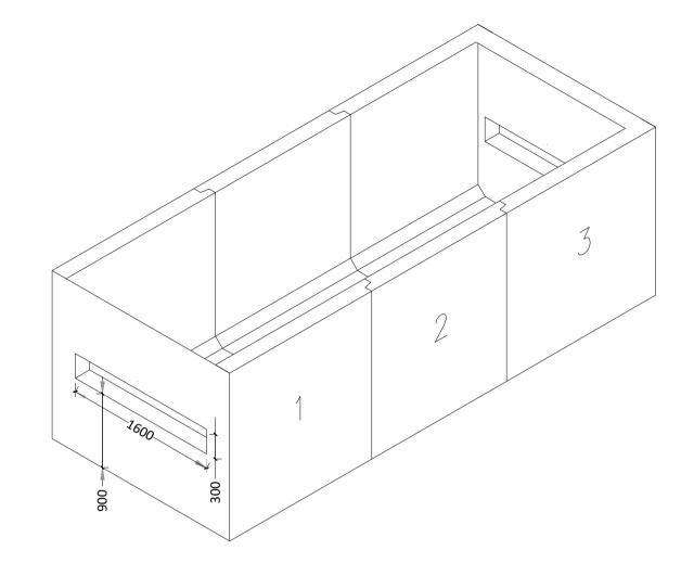
ISOMETRIC VIEW PRECAST CHAMBER
