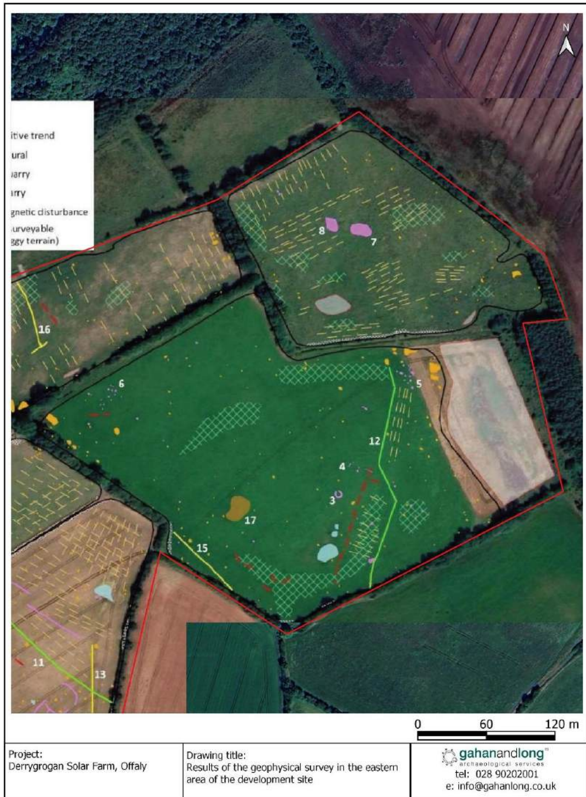
Figure 7: Results of geophysical survey in the eastern area of the development site.
