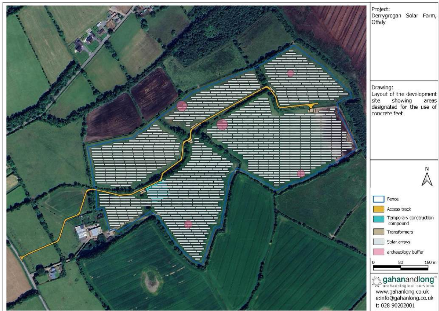
Figure 13: layout of the development site showing areas designated for the use of concrete feet
